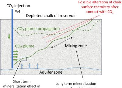
mineralization effect in effect CO<sub>2</sub>/Formation Water contact areas near wellbore
