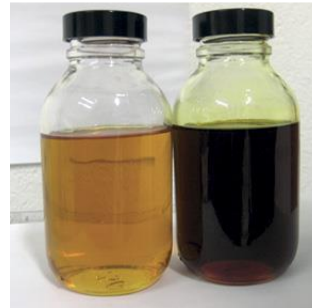
Fig. 2: Degraded hydraulic oil [right] compared to new oil [left] (Source: C.C.JENSEN)
