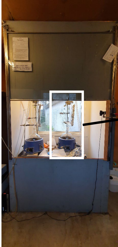
Reflux with toluene to remove oil from pores
