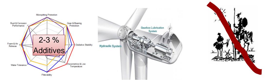
A large turbine contains up to 8000 kg of oily chemicals Inventory in 10000 mills: 80.000 tons
